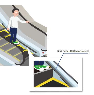
Escalators installed before 1993 might not have been installed with such devices. RPs should consider installing such system in compliance with the requirements of Code of Practice on the Design and Construction of Lifts and Escalators (2012 Edition) - Clause no. 1.1.5.5(c) of Section E Part 4.
