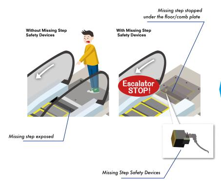
Escalators installed before 1993 might not have been installed with such devices. RPs should consider installing such system in compliance with the requirements of Code of Practice on the Design and Construction of Lifts and Escalators (2012 Edition) - Clause no. 4.5 of Section E Part 4.
