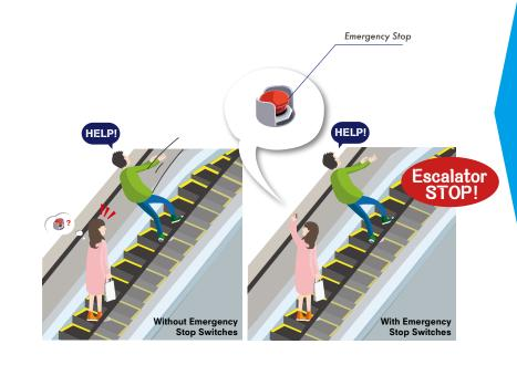
Escalators installed before 1993 might not have been installed with such devices. RPs should consider installing such system in compliance with the requirements of Code of Practice on the Design and Construction of Lifts and Escalators (2012 Edition) - Clause no. 10.3.2.3 of Section E Part 4.
