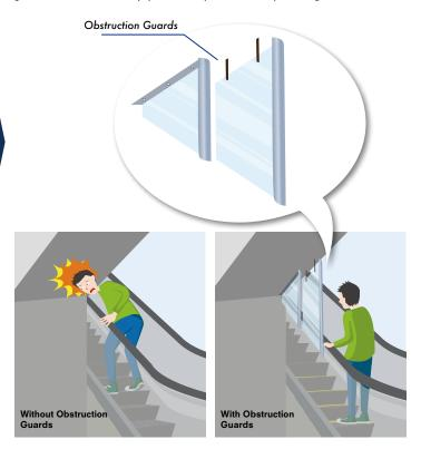
Escalators installed before 1993 might not have been installed with such devices. RPs should consider installing such system in compliance with the requirements of Code of Practice on the Design and Construction of Lifts and Escalators (2012 Edition) - Clause no. 1.2.3 of Section E Part 4.
